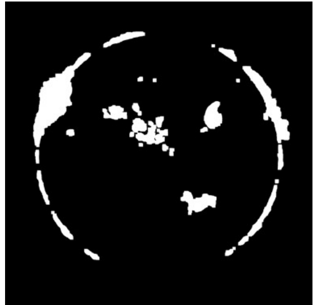
Figure 3. Rough segmentation of active regions for the CBPs filtering after applying the Otsu thresholding and a morphological closing.
