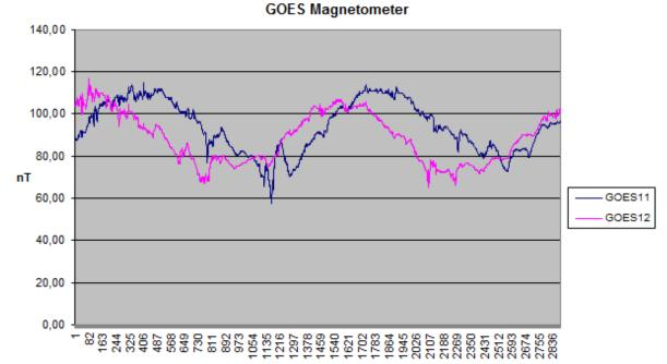
It shows a good example of two correlated timeseries, but with an associated temporal deviation between them. With our prototype tool, it is possible to automatically find the deviation value between them (maximizing the correlation value of the two parameters). This data was obtained from SWENET – Space Weather European Network [1].
